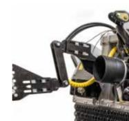
**1 W style self aligning device between PTO drive shaft/gearbox** allows the machine to work at several angles without damaging the PTO
