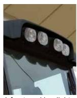
4 front working lights and 4 rear working lights (except B90B: 2 front + 2 rear)
