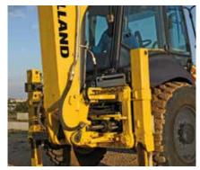
7100 or 110 hp that is 10 hp more than our main competitors! Hydraulic side shift (option):Fast and accurate positioning of theboom without damaging the ground
