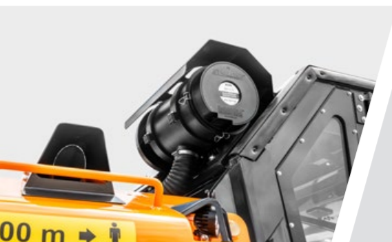
Cabin pressurization system
