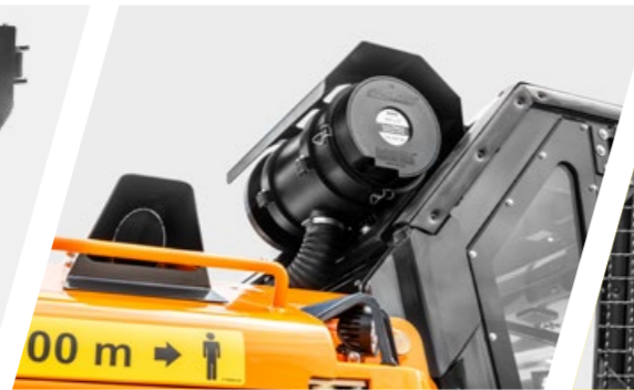
Cabin pressurization system
