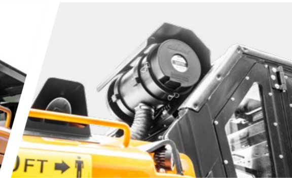
Cabin pressurization system
