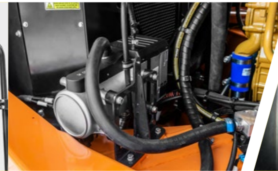
Pre-heating system for engine and hydraulic oil
